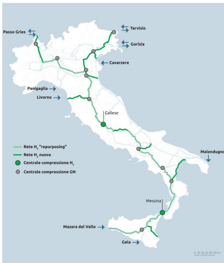
The project concerns the development of a hydrogen backbone that will extend from the entry point in Sicily to the export points with Austria and Switzerland, allowing hydrogen produced in North Africa and Southern Italy to be transported to the main consumption Italian and European consumption areas, which are an integral part of the European hydrogen backbone (EHB).
