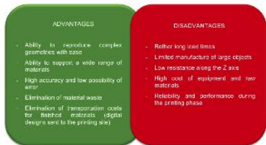
Chart 5 - Advantages and disadvantages of 3D printing method compared to traditional manufacturing of an orthopaedic device.
