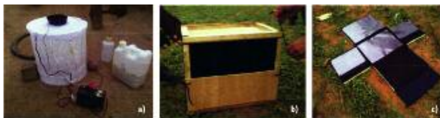
Fig. 1: a) BG-Sentinel trap, triggered with BG-lure (not visible) and CO 2 obtained through yeast fermentation (container on the right); b) Sticky Resting Box closed, triggered with a source of moisture (not visible) and ready to be used in the field and c) Sticky Resting Box open, where you notice the internal adhesive surfaces that act as capture systems.
